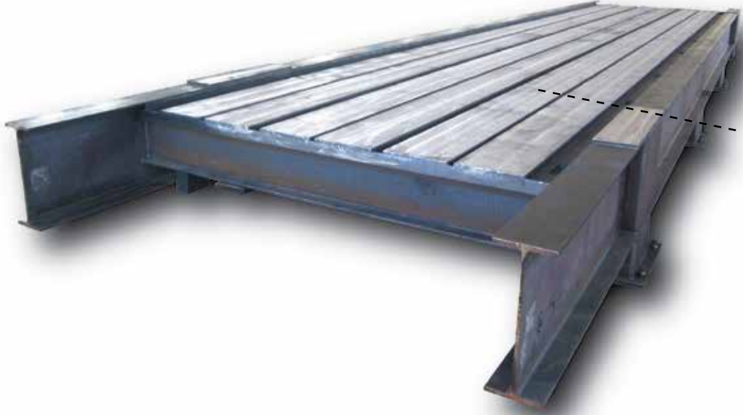
TEK SEFERDE HASSAS FREZELENMİŞ TABLA WORKED IN A SINGLE PIECE ON LARGE-SIZED NUMERICALLY CONTROLLED CENTRES.
